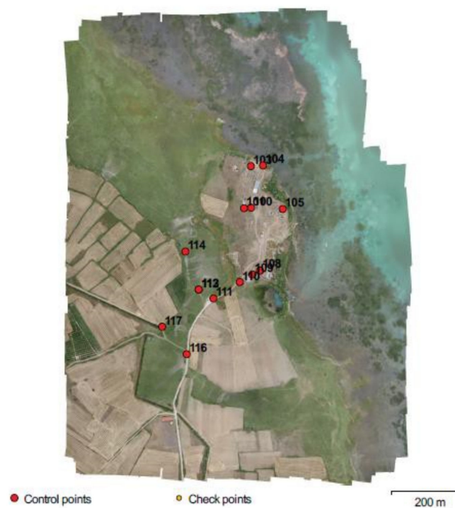
Figure 14. Ground control points.
