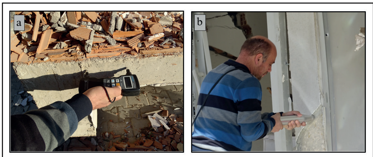
Figure 1. NDT measurements on building concrete
