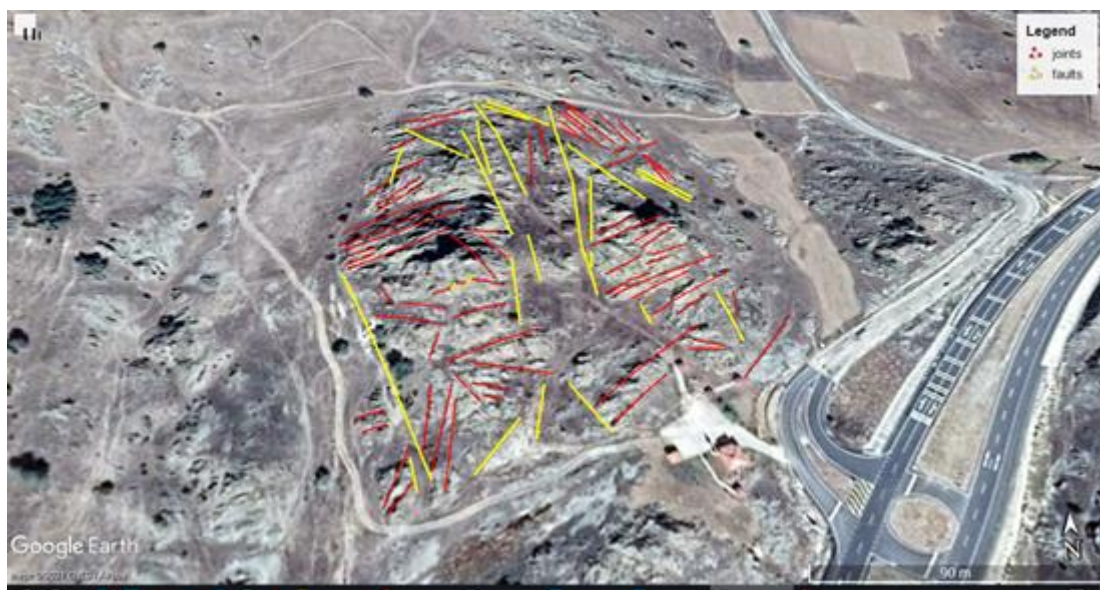
Figure 6: Joint and fault system in plug 4.
