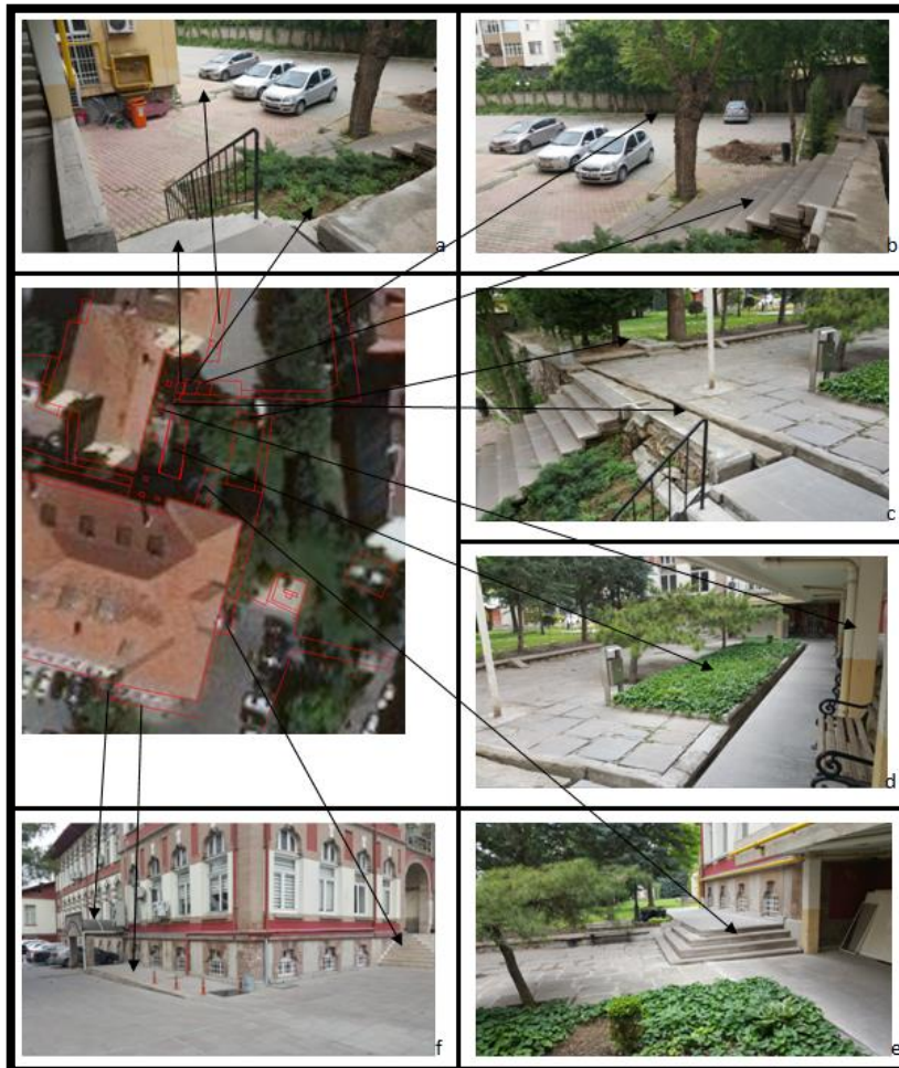
Figure 9. The examples of created polyline objects which define physical obstacles and different types of land use regions that have continuity of internal circulation (Some examples → a: stair, step, pedestrian road, b: stairs, step, landscape area, c: pits, step, landscape area, d: columns, step, landscape area, e: stairs, f: stairs in entrance, pedestrian road, step on pedestrian road,)
