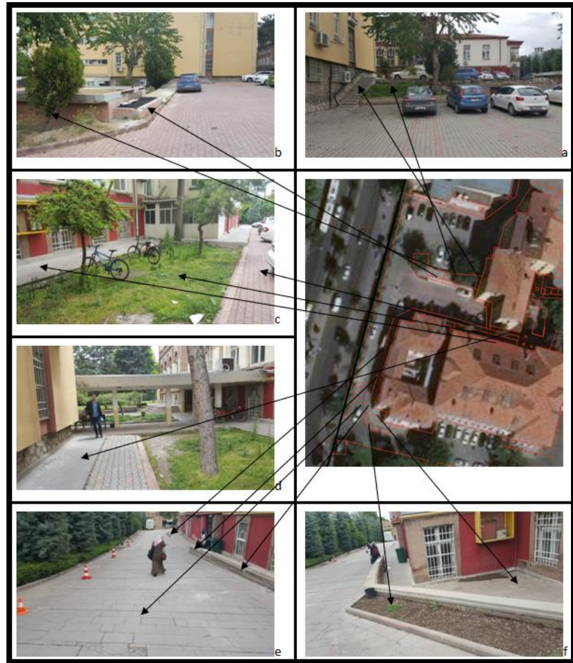
Figure 10. The examples of created GIS based polyline objects which define physical obstacles and different types of land use regions that have continuity of internal circulation in study area (Some examples→a: stairs, wall, landscape area, b: building used for garbage storage, unfitted street furniture on pedestrian road used for ventilation, c: landscape area, pedestrian roads, d: step that separate pedestrian road, e: walls, long steps on vehicle road, f: partial steps, walls, landscape area)
