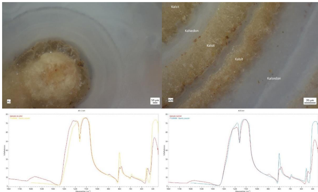
Figure 7. Refractometer graphs of chalcedony and calcite detected in gemology microscope
