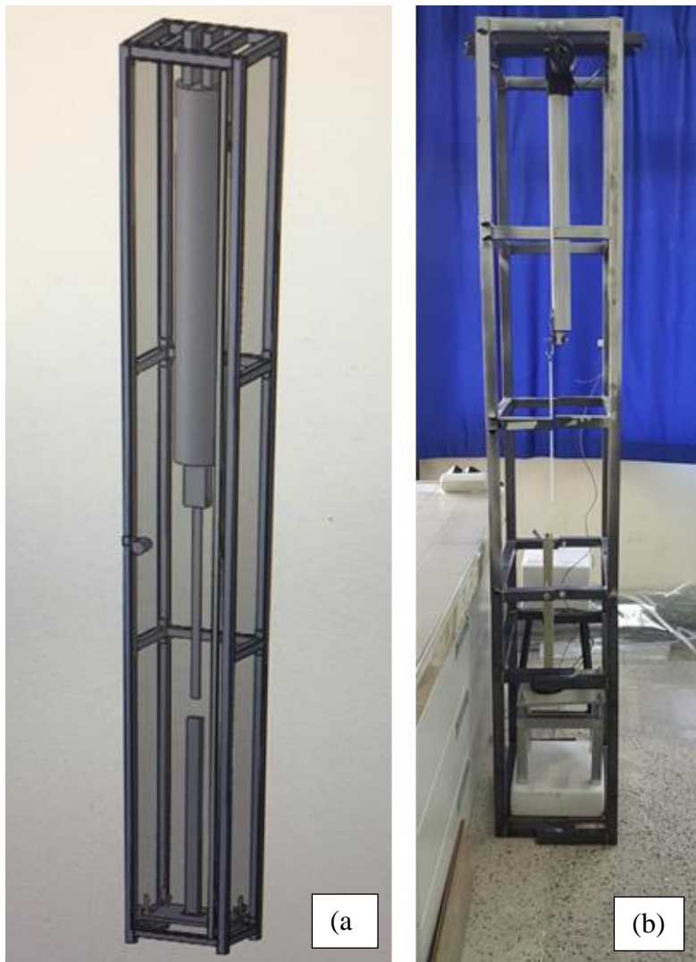
Figure 6. (a) AutoCAD drawing of dip coater and (b) the picture of final device
