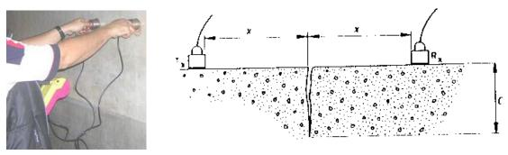
Figure 21. Determination of damage to the building by ultrasonic examination, Source: Aköz and Yüzer, 2009.
