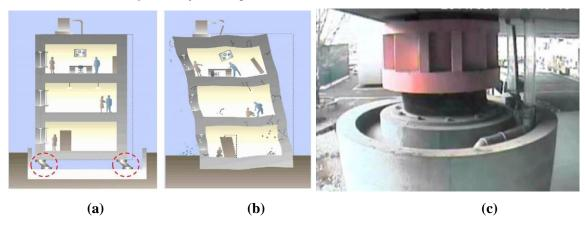
**Figure 10.** (a) Resistance of the seismic isolated structure against earthquake force, (b) Resistance of the structure without seismic isolation against earthquake force, (c) Seismic isolation application in the building, **Source:** Nakamura and Okada, 2019.
