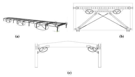
**Figure 13.** (a) Layout of frictional seismic dampers, (b) Inverse V type friction seismic damper placement, (c) Corner junction friction seismic damper placement, **Source:** Yıldırım and others, 2015.
