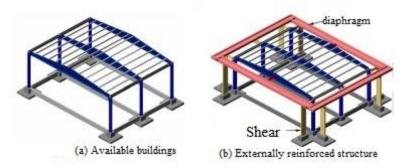
**Figure 14.** Building models reinforced with external shear diaphragm with the existing structure, **Source:** Kaplan and others, 2009.
