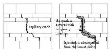
Figure 9. Injection repair of small cracks, Source: Aköz, 2008.
