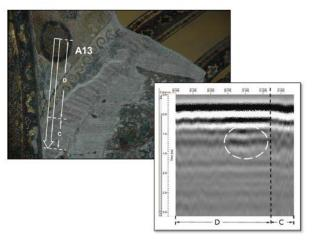
**Figure 20.** GPR scan of the mosaic area unearthed in Hagia Sophia (The target shown by the dashed white curve corresponds to an interior space filled with mortars and bricks), **Source:** Moropoulou and others, 2013.
