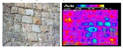
**Figure 19.** Left: Walls facing the National Heraklion Stadium in Crete; Right: Infrared thermography of the same wall, **Source:** Moropoulou and others, 2013.
