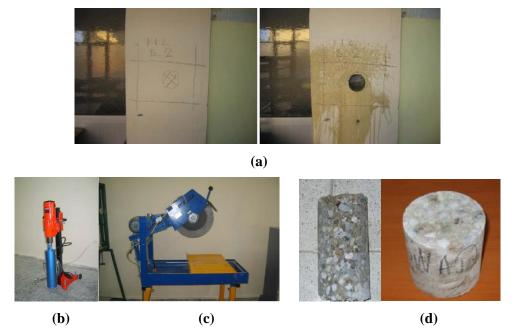
**Figure 16.** (a) Taking the core sample to determine the compressive strength of concrete, **Source:** Kanıt and Altın, 2008, (b) Coring tool, **Source:** Altın 2008, (c) The tool used for cutting the core, **Source:** Altın 2008, (d) Extracted and cut core samples, **Source:** Altın 2008.
