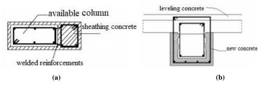
**Figure 1.** (a) Jacket strengthening plan of the column, (b) Strengthening section of the beam, **Source:** Gülmez, 2010.
