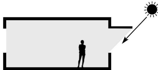
Figure 8. Cooling via shading elements
