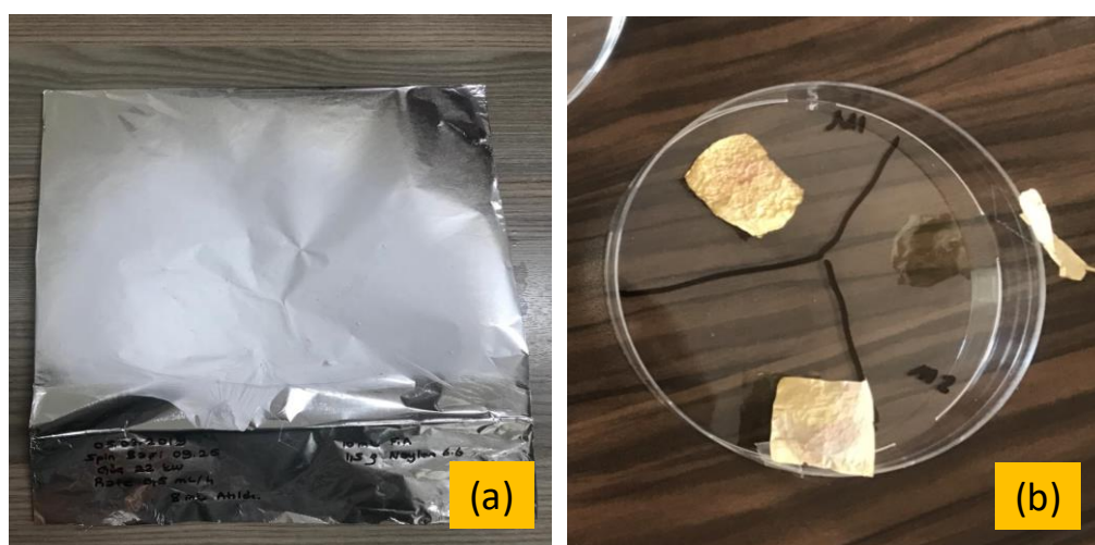
Figure 1. Electrospun Nylon 6,6 nanofibers and modified nanofibers with AgNPs
