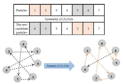
Figure 5. The symmetry method
