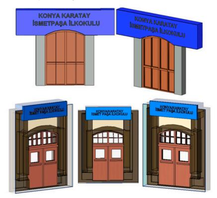
detailed door drawings. Figure 14 depicts a shaded view of the model built by including the door object drawing in the 3D model.
