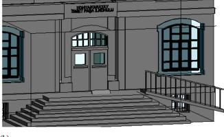
**Figure 15.** Manual drawing of stairs, ramps, and railing objects. (**a**) stairs and railing details and (**b**) entry ramp and staircase object.
