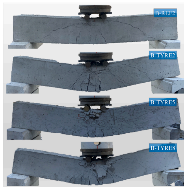
Fig. 6. Failure patterns of tested beams – II.
