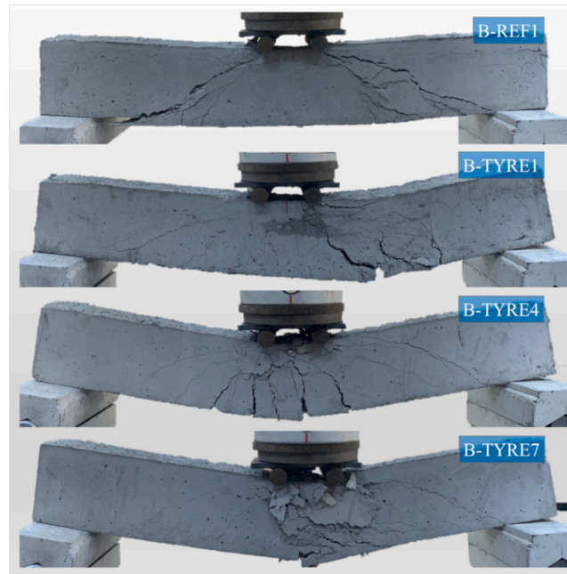
Fig. 5. Failure patterns of tested beams – I.
