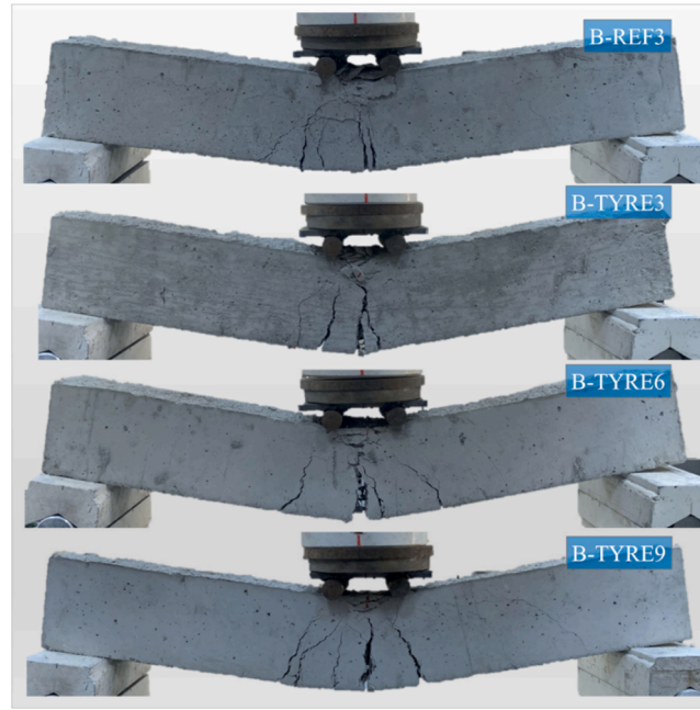
Fig. 7. Failure patterns of tested beams – III.
