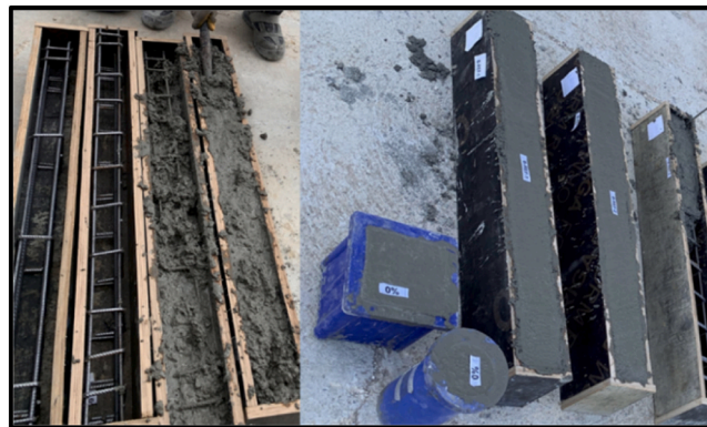
Fig. 2. Preparation of beams.
