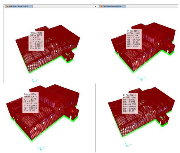
Figure 9. Maximum displacement under G+EX G+EY loading (mm) for DBYBHY 2007 and TBDY 2018
