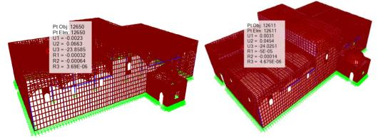
Figure 8. Maximum displacement under G loading (mm) for DBYBHY 2007 and TBDY 2018
