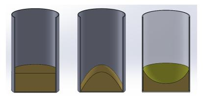
Figure. 1 Grain surface condition types in silo (a) levelled (b) peaked cone (c) inverted cone
