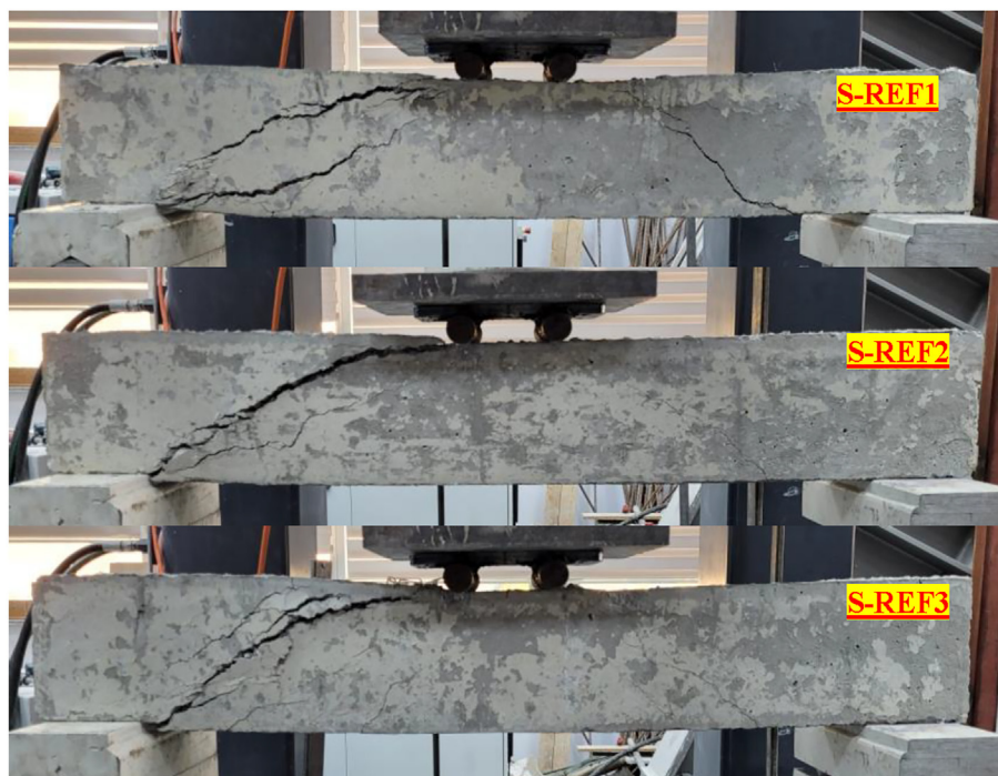
Fig. 5 – Fracture and shear behavior of RCB for S-REF1, S-REF2, S-REF3.
