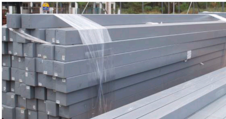
Figure 2. Cross-arm beams in stockpiles after pultrusion for distribution [57].
