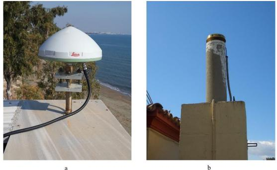
Figure 1. MERS (a) and EBRE (b) stations used in the application (https://igs.org/network/)
