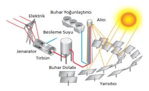
Figure 1. Concentrated solar energy systems (CSP)
