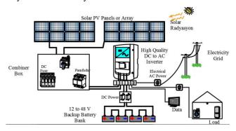
Figure 4. On-Off Grid Network
