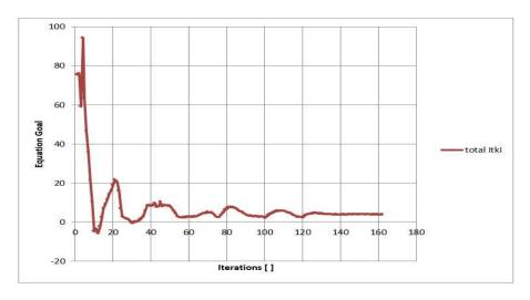
Figure 3. Graph of thrust force when thrusters are fed by 16V
