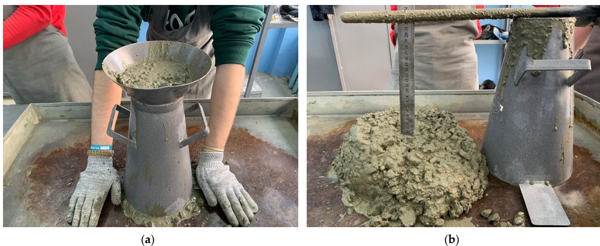
Figure 4. Testing the concrete mix for workability: (a) filling and bayoneting the mix in a cone; (b) slump measurement.
