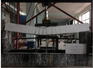
Figure 10. Fractures in specimen (B-3)
