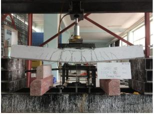
Figure 7. Fractures in specimen (B-2)
