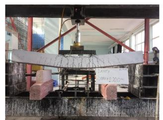
Figure 14. Fractures in specimen (B-8)
