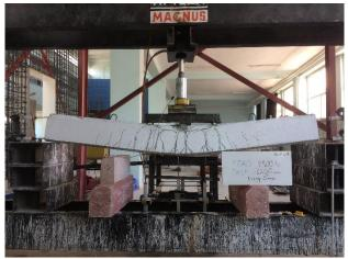
Figure 13. Fractures in specimen (B-4)
