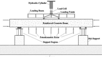
Rigid Slab Figure 1. Test Setup
