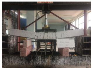
Figure 8. Fractures in specimen (B-6)
