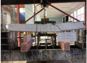
Figure 4. Fractures in specimen (B-1)
