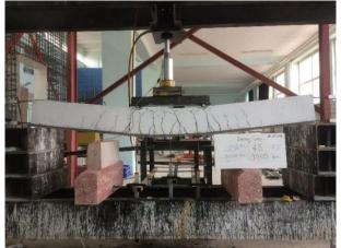
Figure 5. Fractures in specimen (B-5)
