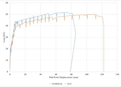
Figure 6. Load- Displacement Curve (B-2 and B-6)
