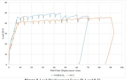
Figure 3. Load-Displacement Curve (B-1 and B-5)
