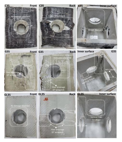
Figure 9. Damage analyses of C35, G35, and GL35.
