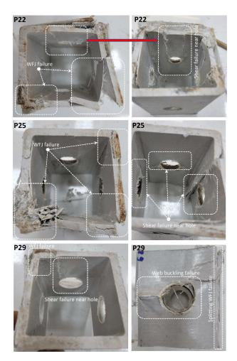
Figure 6. Damage analyses of P22, P25, and P29.
