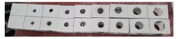
Figure 2. Specimens with different opening sizes.
