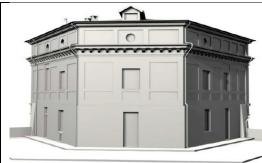
**Figure 8.** 3D model of building, created by using point cloud (GECO Lab.).
