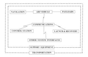
Figure 2. UAV system – functional structure (Austin, 2010)
