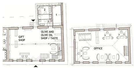
Figure 15. Ground floor plan of shop and service building Figure 16. First floor plan of shop – office
