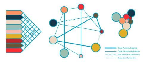
Figure 3.4. Relationship matrix, starting configuration and one possible layout
