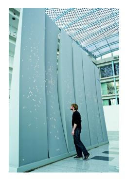
Fig 01. The skin of each InteractiveWall covered by a unique, irregular distribution of dynamically controlled LED's that form a highly reactive interface.
