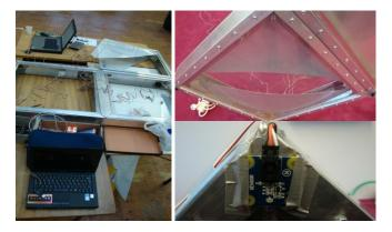
Fig 09. View showing the assembly details of the actuators and motors on the internal frame of the prototype and the mounting of touch sensors on the external frame of the prototype.
