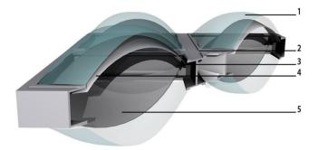
Fig 08. View showing the internal structural make-up of the sandwich component. The ETFE sheets (1) are inflated and connected to the C profiles (2) along their perimeter. The pointer (3) shows the connection point between one of the movable extremities and the small rail in aluminium (that is welded to the C profile). The two movable membranes (4, 5) have a triangular shape and assume two opposite curvatures during their movement.
