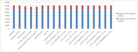
Figure 15 Heating and cooling consumptions of scenarios
