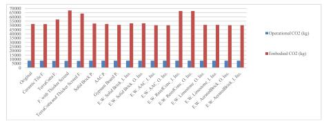
Figure 16 Embodied and operation carbon emissions of scenarios
