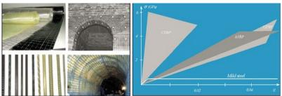
Figure 2. FRP applications and stress-strain relationships (Beg et al. 2006)
