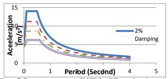
Figure 7. Response spectrum of MCE for different damping ratios
