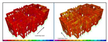
Figure 11. S11 stresses under MCE for isolated Beylerbeyi Palace with HDRB
