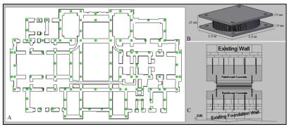
Figure 13. Details of HDRB application in Beylerbeyi Palace
