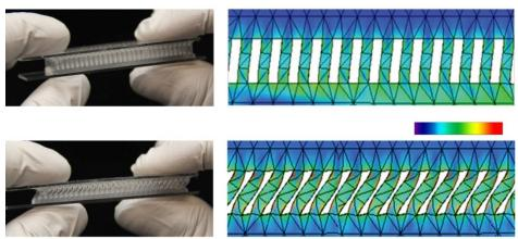
Figure 2: The patented Dynamic Daylight Control System, a joint development of designers and scientists, relies on the shearing of soft pneumatic layers to control daylight<sup>2</sup>.
