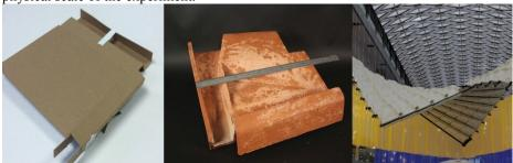
Figure 5: Prototyping at different levels of precision was key in developing a novel ceramic structure.<sup>1</sup>
