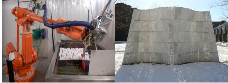
Figure 1: Robotically waterjet, stone slabs were manipulated such that 72 perforated thin stone slabs, precisely cut, could be dry-assembled into a loadbearing and post-tensioned shell.
