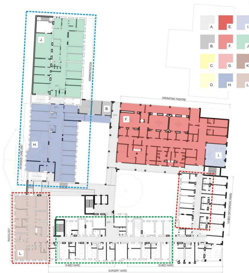
Figure 5. New hospital lay-out as designed, 1st floor; key: A – communication, B – magazines, F – operating theatre, H – intensive care unit, I – observation unit, J – administration, L – radiology; green dashed line – first building, red dashed line – 1930s extension, blue dashed line – 1970s and 1980s extension
