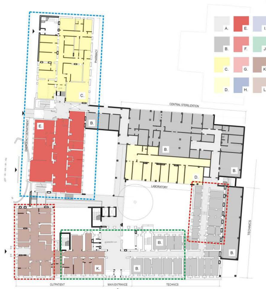
Figure 4. New hospital lay-out as designed, ground floor; key: A – communication, B – technics, magazines, C – pharmacy, D – laboratory, E – emergency department, K – outpatient; green dashed line – first building, red dashed line – 1930s extension, blue dashed line – 1970s and 1980s extension
