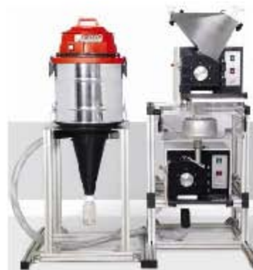
Figure 7. The chopping machines is directly linked and integrated with the collector and dust absorber, avoiding the dust clouds. Machine is supported by
