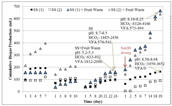
**Figure 3.** Cumulative biogas production and pH/HCO<sub>3</sub>·/VFA in SS digestion with and without fruit waste (HCO<sub>3</sub>·/VFA concentrations in mg CaCO<sub>3</sub>/L)
