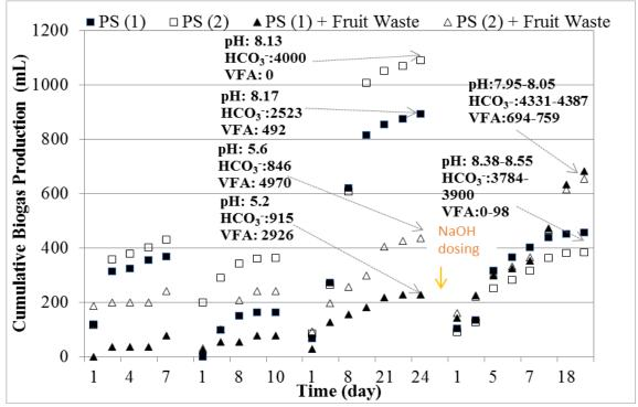
**Figure 2.** Cumulative biogas production and pH/HCO<sub>3</sub>-/VFA in PS digestion with and without fruit waste (HCO<sub>3</sub>-/VFA concentrations in mg CaCO<sub>3</sub>/L)
