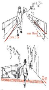
Figure 4. Railing dimensions.
