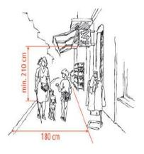
**Figure 1.** Pavement Widths and Hung Obstacles Dimensions.
