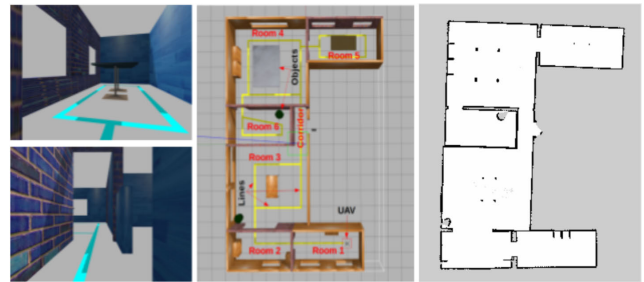
FIGURE 3. Simulation environment, its 2D grid map and sample camera views of Tello UAV.
