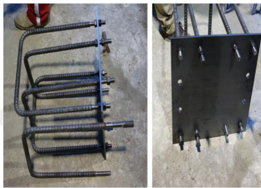
(a) Fabricated C-type re-bars for experiment
