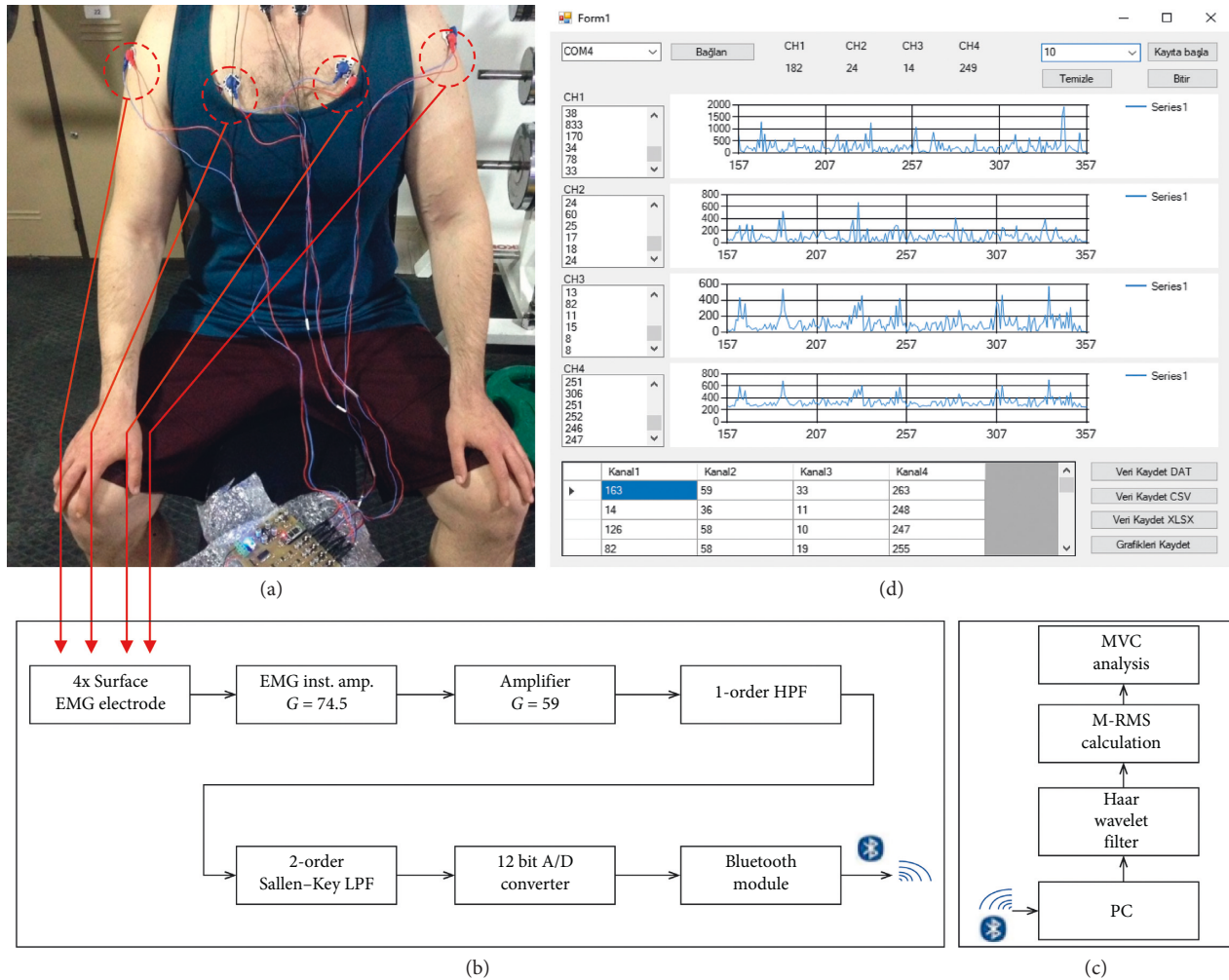
FIGURE 3: Overview of the system. (a) Connecting electrodes before training (Photoshoot by Orucu). (b) Block diagram of the SEMG circuit. (c) Block diagram of the analysis software. (d) User interface of the analysis software.
